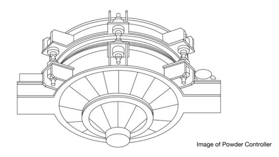
The bridges are broken by the circular motion of the lower part so that the material is discharged constantly. Depending on the properties of the powder, the discharge amount can be adjusted by changing the number of vibrations with an inverter.
